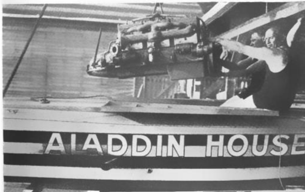
One of the Scripps' Motors with which all the boats were powered, being lowered into one of the racing craft, by Ned and Bob Purdy, who designed and built all of them.
