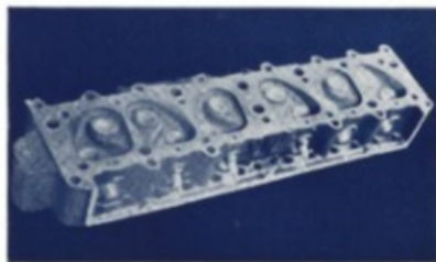
Illustration shows clean condition of cylinder head after 5000 miles run.
