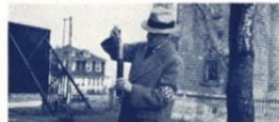
H. H. Allen determining the specific gravity and temperature of a sample of the oil drawn from the crankcase after the test.
