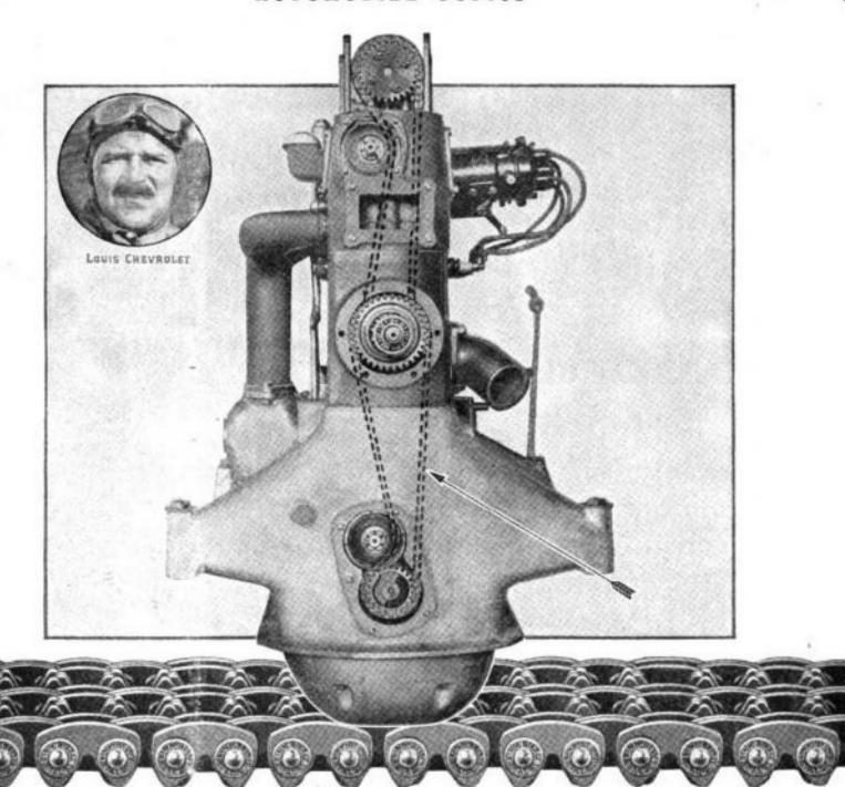
Louis Chevrolet, the intrepid designer-driver, determined upon the Link-Belt silent chain drive and Link-Belt automatic tightener for the "front end" of his new Frontenac engine. Two chains and two automatic tighteners are used.
