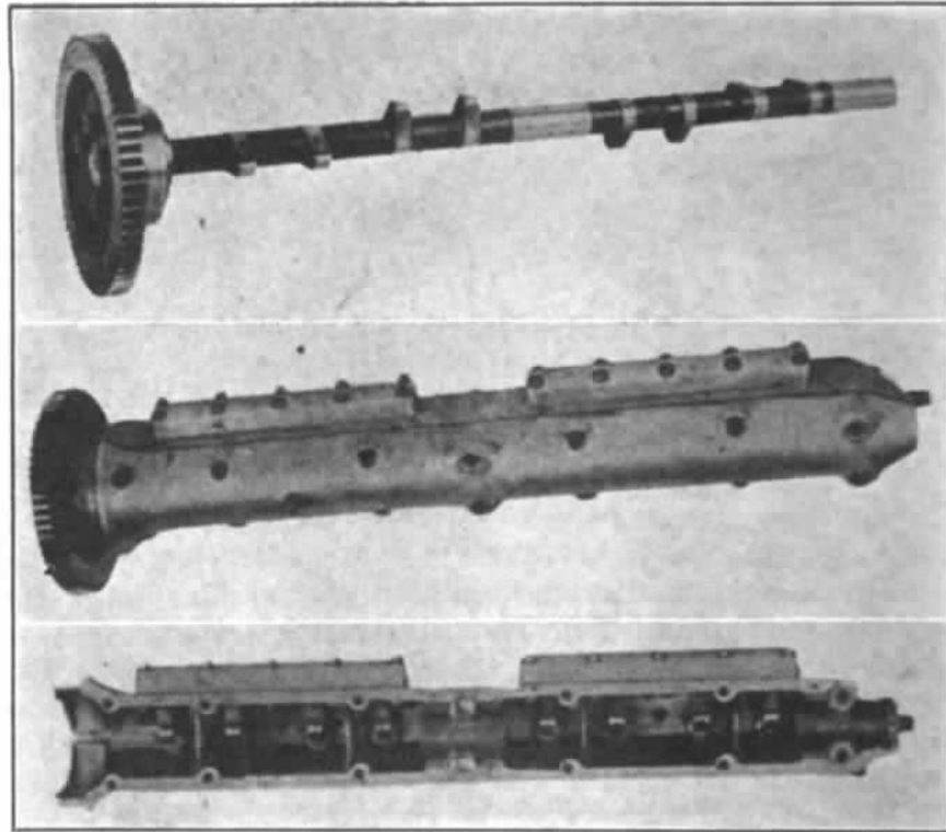
FIG. 4—ONE OF THE CAMSHAFTS AT THE TOP WITH THE COMPLETE CAM HOUSING UNDERNEATH AND AN INTERIOR VIEW OF THE HOUSING WITH THE BRONZE CAPS FORMING CAMSHAFT BEARING AT THE BOTTOM
