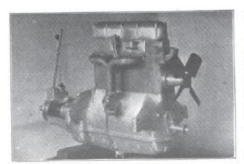
SOME clever engineering is evidenced in the cleancut design of the Frontenac engine. On the right side of the engine will be noted the oil filler. On the left side are the carbureter and distributor
