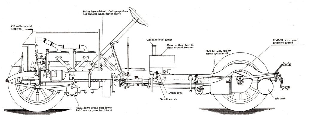
Keep all grease cups (marked in red) filled up—use good graphite grease
