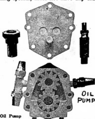
Oil Sump and Oil Pump
